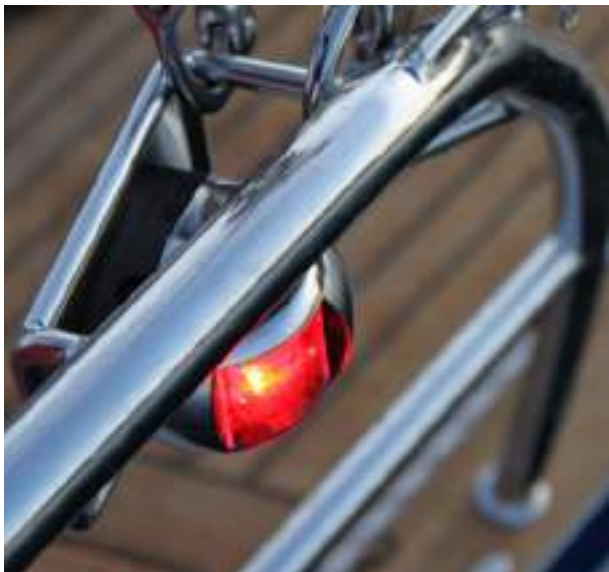
The LED navigation lights with low power consumption are so positioned that they are not easily damaged
