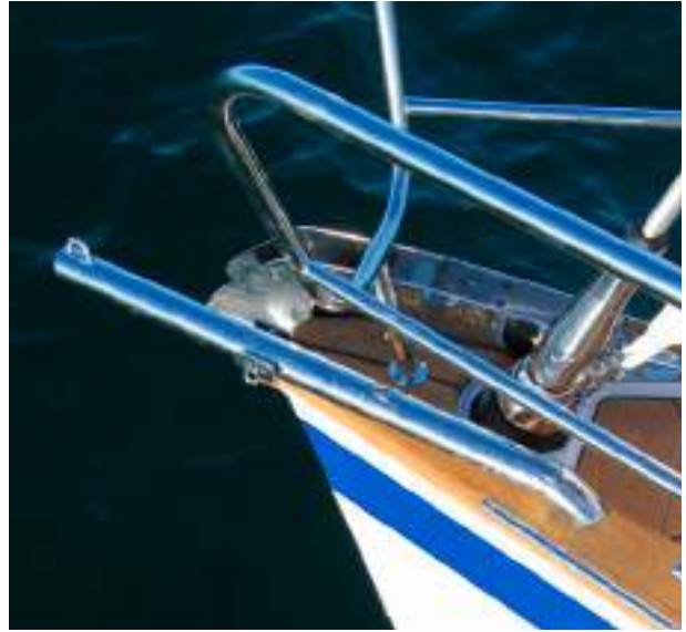
Optional removable gennaker / code zero bowsprit with optimized sail
