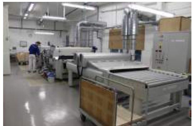
Fully automatic varnishing machines
