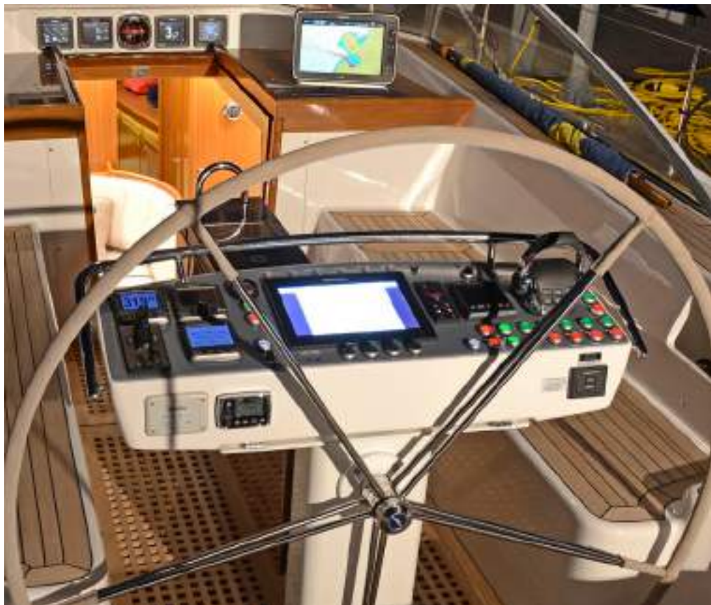
Push-button controls for "everything" on the steering pedestal
