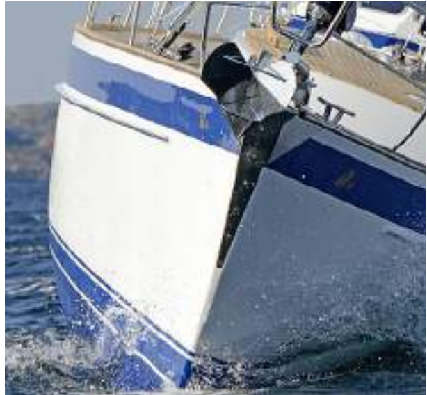
A sturdy rubbing strake is integral to the hull
