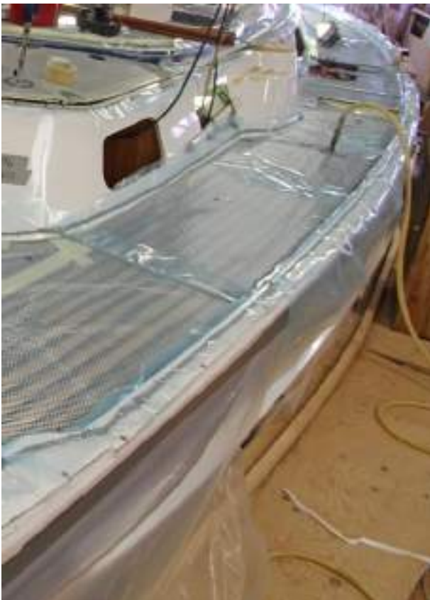
Completely vacuum glued teak decks, no screws at all
