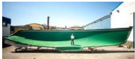
The port side of the Hallberg-Rassy 64 hull mould
