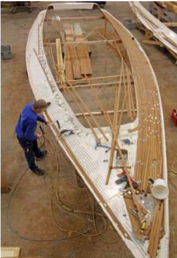
Teak deck, handcrafted on a template outside the boat, 10 mm thick solid wood, completely vacuum glued without screws to the GRP deck for long service life
