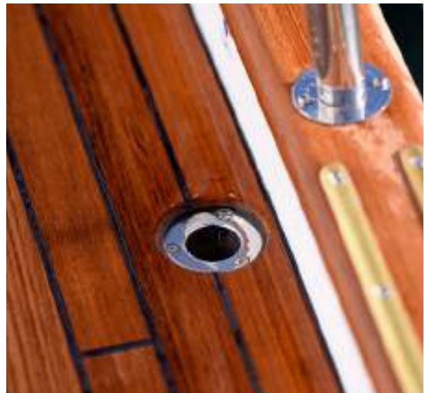
Deck drains with exits under the waterline, to prevent stains on the hullside
