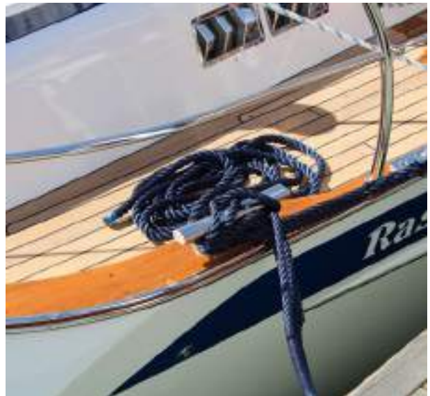
Sturdy stainless mooring and spring cleats, secured with four bolts each
