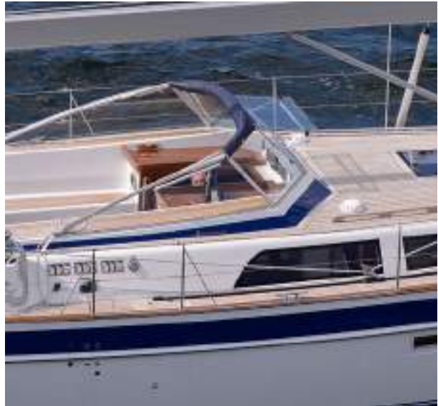
An opening mid section in the wind screen gives good ventilation
