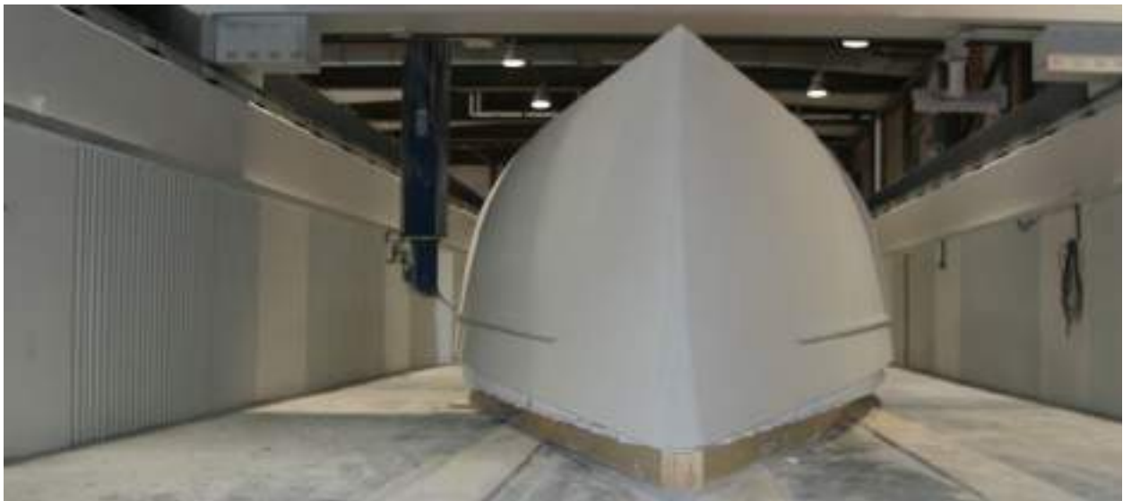
The plug takes shape in a CNC milling machine
