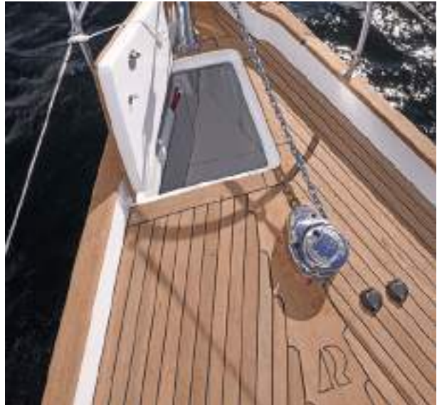
Asymmetric chain locker opening makes it possible to step to the very front of the boat even if the chain is moving
