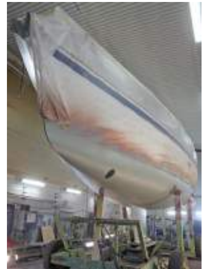
Two coats of epoxy primer and two coats of antifouling applied as standard
