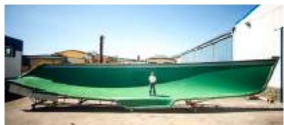
The port side of the Hallberg-Rassy 64 hull mould
