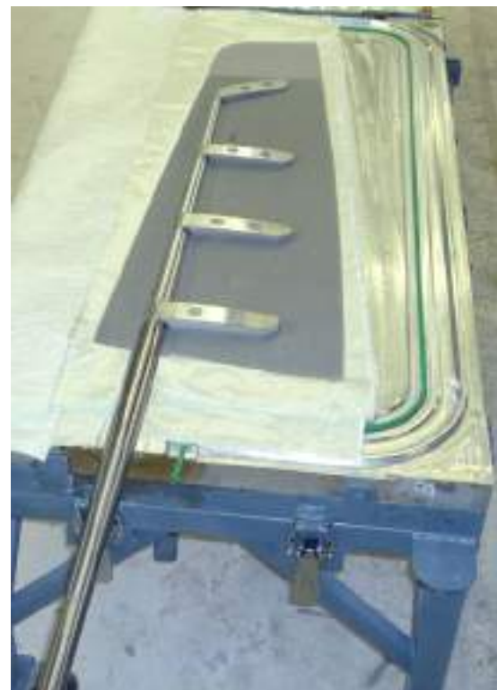
The rigid rudder has a solid stainless shaft (no pipe) that is moulded into the solid rudder blade
