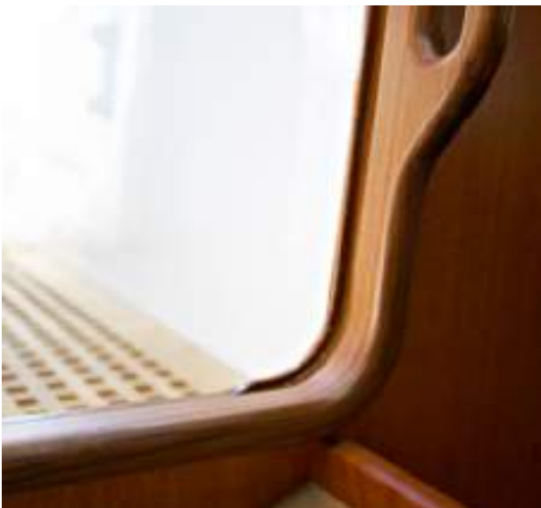
The entrance frame is moulded of veneers in one piece
