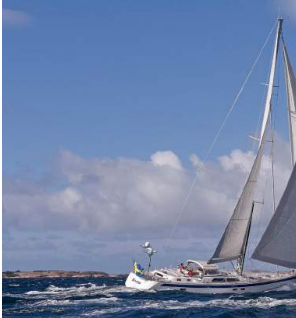
Above: two Hallberg-Rassy 64's with sails hydraulically furled and reefed from push-buttons at the steering stand; the winches are also powered. A mere fingertip movement controls even the biggest yacht
