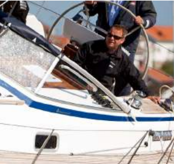
A handhold in the windscreen offers good safety when stepping in or out of the cockpit
